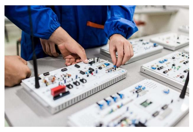
The laboratory includes various modules to show and experiment circuits and principles commonly recurrent in the field of telecommunications. As such, this laboratory is recommended for students attending any subsequent communications speciality. The modules generally consist of PCB cards with components in view, especially suitable for individual student work or work in a small group.
